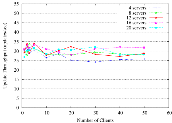
Figure 21: Paxos-complete Throughput, Synchronous Disk Writes
